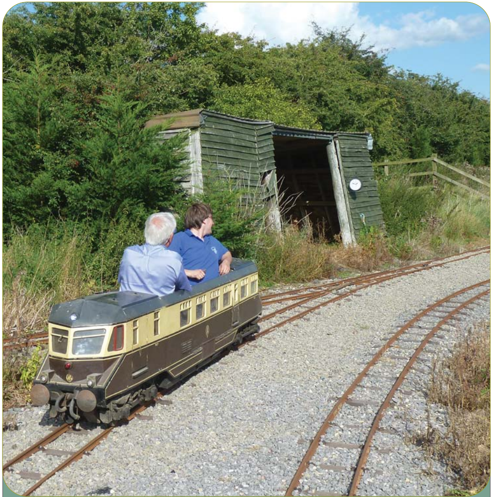
Bob's GWR railcar 'Monica' was another delightful machine, built in 2004 by Jim Rough. Like the tank loco, it came to the Grittenham Light Railway in 2013, and it was re-engined from petrol to diesel while it was there. It could carry two at a pinch, but it was cosy, and clearly a rather uncomfortable arrangement! The railcar has just left the main station heading north and approaching the cattle grid, with roughly 500 metres still to go, to complete the circuit
